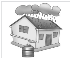
Rooftop rainwater harvesting
